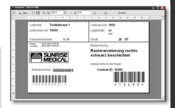
These groups are different regarding the processes. But they are based on the same principle: If an operator is taking out the last part from a Kanban box the Kanban container has to be scanned to the status EMPTY via barcode reader. The empty Kanban box is the signal to start the internal production of the parts or for the external supplier to deliver a new re-filled box (PULL).
